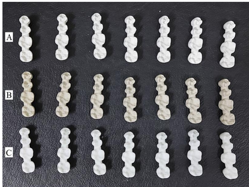
Figure 3: The completed frameworks (A)PEEK, (B)PEKK, (C) Sintered Zirconia
