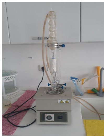
Figure 2: Soxhlet extraction of fungi samples
